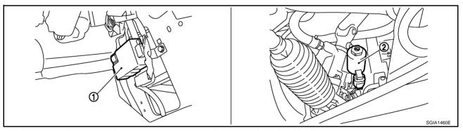
Power steering control unit (Back of dash side finisher RH)
