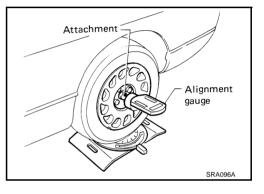
If outside the standard value, adjust with adjusting bolt in front lower link.
